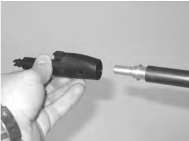
Repeat the process for the removal of the other rivets, so the upper swivelling part can be removed.
