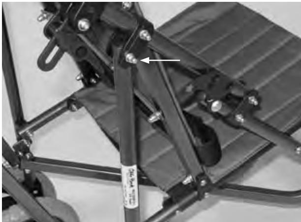
Loosen and remove the screw connections between the posterior frame and the push handle.
