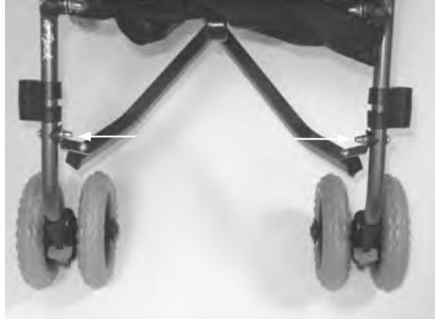
Loosen and remove the screw connections between the anterior frame and the folding scissor construction.
