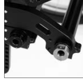
MG 85 Wheelbase extension with second axle
