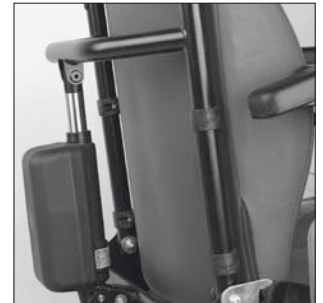
ED 50 Electric back angle adjustment 30°
